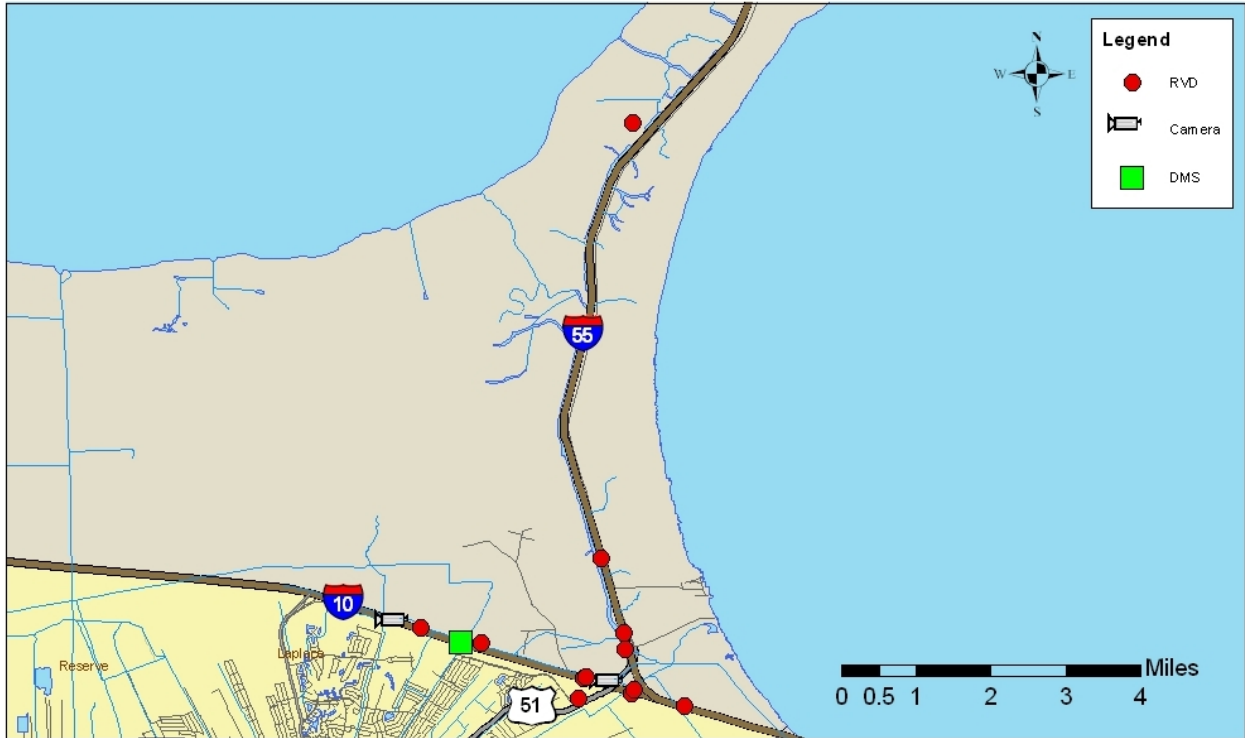
Figure 4a: Existing LADOTD ITS Equipment Within Project Limits
